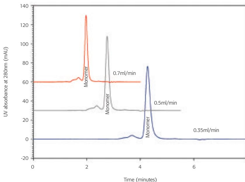
High-performance size-exclusion liquid chromatography (SEC) on silica-based columns is the industry's standard technique for separating and quantifying soluble protein aggregates – an analysis which is always required for regulatory approval.
