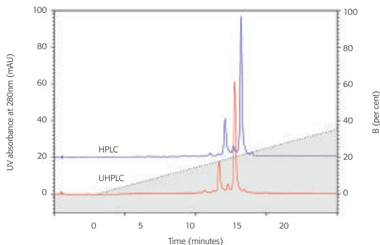
**Figure 1b:** Zoomed elution profile of the mAb charge variants on TSKgel SP-STAT. The zoom provides better insights into what extent the elution profile benefits from using a UHPLC system. The peak width is smaller for the UHPLC elution profile, compared to the HPLC chromatogram. Due to the decreased system dead volume, peak elution occurs earlier than for the HPLC system
