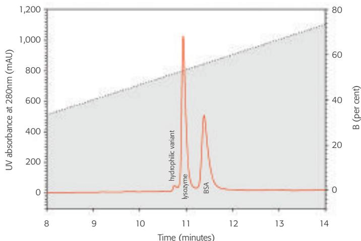
**Figure 3b:** Exchanging the UV flow cell to a semi-micro 2.5µL flow cell led to an increase in resolution of the two proteins by approximately 25 per cent when applying the same conditions
