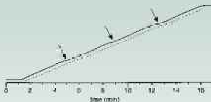
Figure 9. Plot of linear gradient with faulty proportioning valves. Arrows show deviations from linearity; dashed line drawn below plot for reference. Gradient 0 – 100% B in 15 min at 1 mL/min; A = water, B = 0.1% acetone in water; detection UV 265 nm. Adapted from [4].
