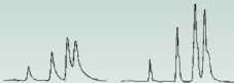
Figure 3. Peak distortion of all peaks in the chromatogram due to a partially blocked frit or column void.
