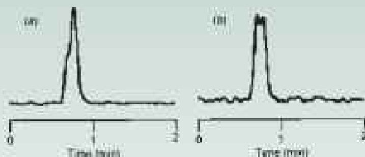
Figure 4. Split peaks due to the presence of a second component. (a) 25 ng/mL, and (b) 10 ng/mL of drug (second peak) in plasma. Adapted from [1].
