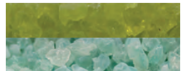
CoFree™ Adsorbent: Top: Full Capacity; Bottom: Depleted.
