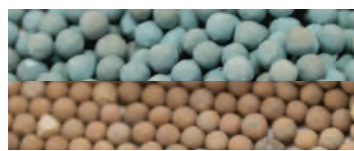
H 2 O Adsorbent: Top: Full Capacity; Bottom: Depleted.
