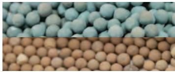
Moisture Adsorbent: Top: Full Capacity; Bottom: Depleted.
