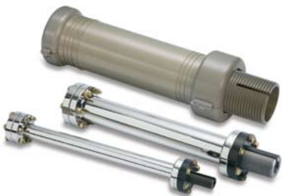
MODcol® Dynamic Axial Compression Spring® columns are the only mobile DAC columns on the market. They can be used without being mounted in the Multipacker® instrument with full DAC functionality. The Spring® columns are available in 1", 2" and 4" i.d. and 2 lengths, which enable packed bed lengths from 15–30cm.
