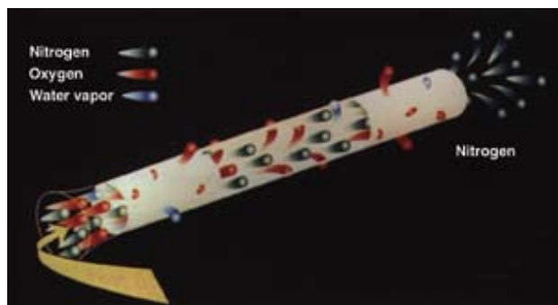
Water vapor and oxygen permeate through the wall of the membrane quickly. Only nitrogen flows through the fiber bores to the ELSD.
