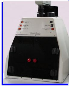
The hoods of the RH-5 series all provide a built-in UV transilluminator with a filter size of 22 x 28 cm (8.7 x 11 inches) on a pull-out rail.
