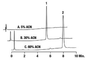
Column: Mobile Phase: Gradient:  $\label{eq:c4} Vydac \& C4, 5 \mu m, 50 \ x \ 4.6 mm \ (Part No. 214 TP 5405) \\ A: 0.1\% \ Trifluoroacetic Acid B: Acetonitrile$
