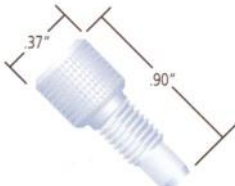
UP-P-100 1/14-28 Kel-F™ Fitting for 1/8" OD tubing Max Pressure 69 bar
